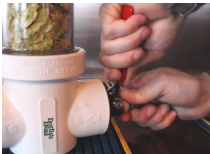
Figure 7: Attaching Other End of Hose to Randall Inlet Shank
